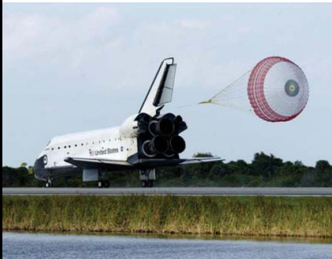
Shuttle Endeavour's drag chute slows down the as it lands on runway 33 at the SLF.
