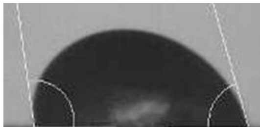
Fig 4. Droplet and contact angles.
